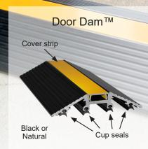
Cleverseal Door Dam Threshold Seal provides a tight, long lasting barrier to prevent water pooling inside your garage. The ground-breaking design of Cleverseal Door Dam is made of hard-wearing aluminium with the additional protection of four bottom PVC cup seals, that compress against the garage floor to provide an immediate tight seal to stop water soaking your garage floor.
